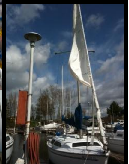
Always secure your roller furling sails or you might have one end up like this. On an eventful Saturday last month our weather station clocked the wind at 47 kts.
